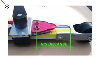
**Mounting NIS rollerski plates:** Measure to the center of the heelplate holes! Adjust the shoesize at the jig.
